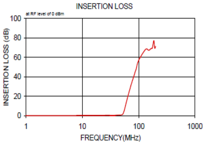
Insertion loss of Filter.
